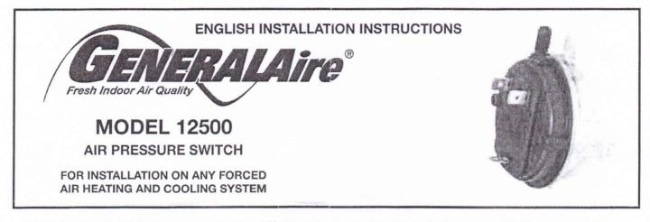
This Air Pressure Switch is designed to control Humidifier operation by sensing changes in air pressure within the furnace plenums when the furnace is in operation. The Air Pressure Switch can be actuated by a positive pressure, negative pressure or a differential pressure of .05" W.C. or more. The Air Pressure Switch contains normally open, single throw contacts to complete the humidifier control circuit or supply 24V A.C. to the humidifier when the furnace blower runs.
